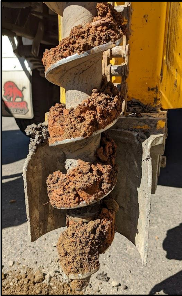
Figure 17. Drilling of BH10. The soil is silty clay and dry.
