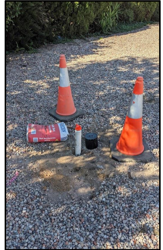
Figure 19. An example of groundwater monitoring wells (MW3) installed within the site.
